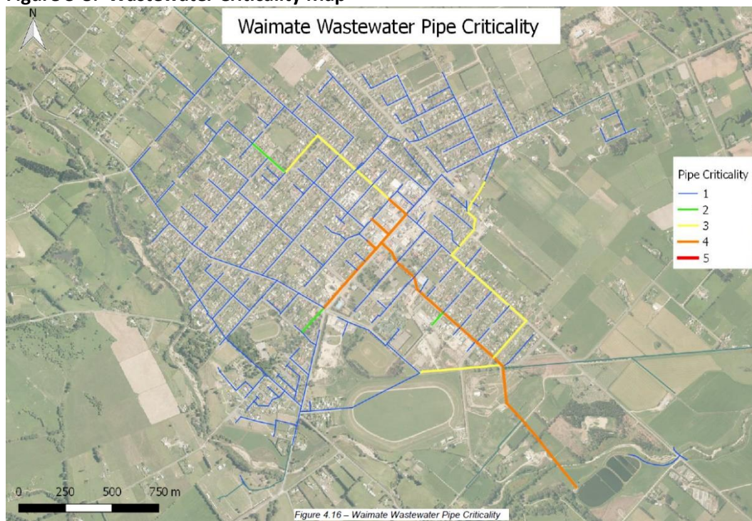
Figure 3-8: Wastewater Criticality Map
